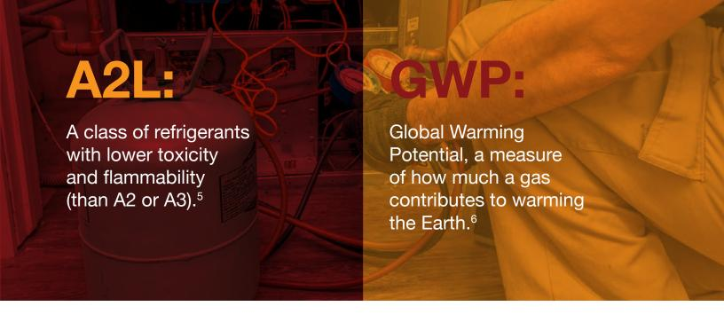
Many replacements for R-22 or alternative refrigerants have high GWP. For instance, 410A has a GWP of 2,088,<sup>7</sup> which means the warming potential of one pound of 410A released into the atmosphere is more than 2,000 pounds of Carbon Dioxide (CO<sub>2</sub>).
